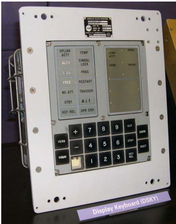
FIGURE 1: THE DISPLAY KEYBOARD OR DSKY OF THE APOLLO GUIDANCE COMPUTER
